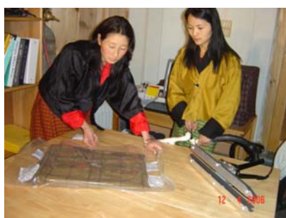
Figure 1. Removing oxygen from film bag with vacuum and Y hose
