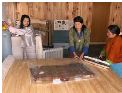
Figure 3. Purging the barrier film with nitrogen
