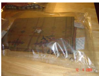
Figure 5. The finished film bag with Ageless packets and eye
