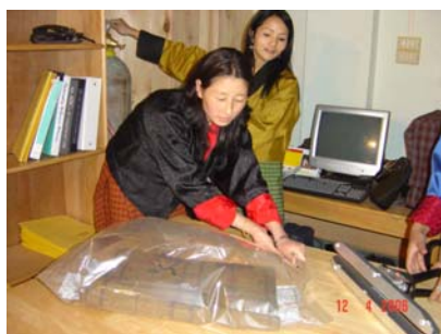
Figure 2. Purging the bag with nitrogen
